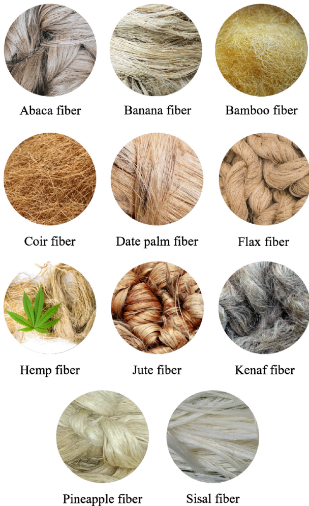
Fig. 1. General plant fibers used in the automotive biocomposites [22-32]
