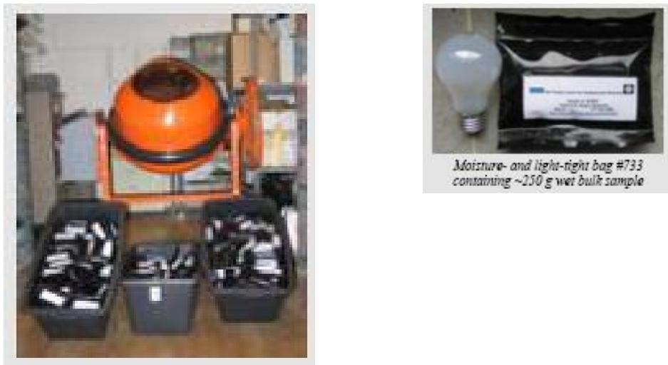
Figure 3. Mixing machine for homogenization of samples and measurement samples distributed to each laboratory (Buylaert *et al.*, 2011).
