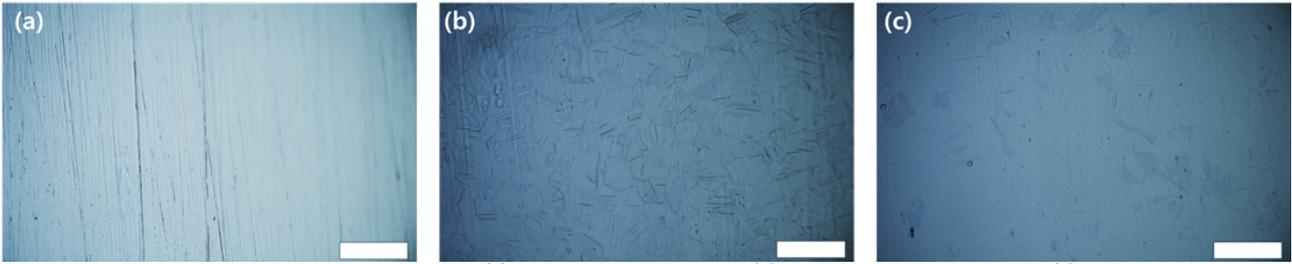
Fig. 2. Surface topology of STS 304 sample (a) non-electropolishing (b) electropolishing 15 min (c) electropolishing 25 min. Scale bar is 70 μm
