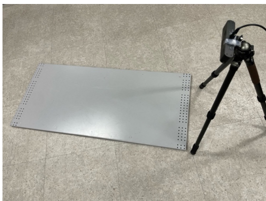
Fig. 4 Installation of a ZED stereo vision camera and prefabricated steel structures
