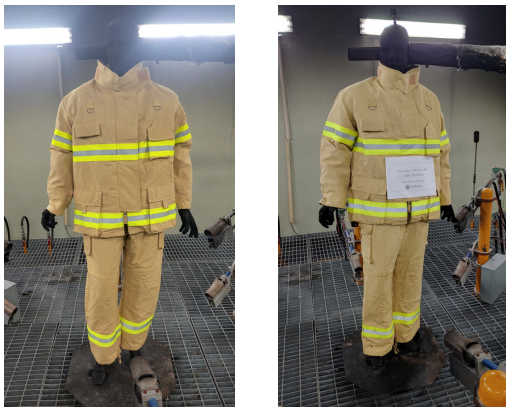
(a) Mannequin unusing SAP (b) Mannequin using SAP Fig. 6. Mannequins in the full-scale thermal exposure tests
