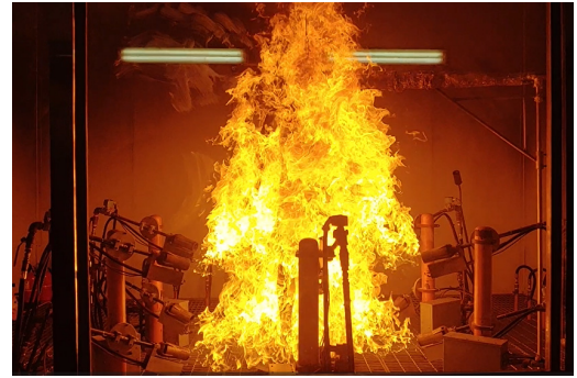
Fig. 3. Mannequin flame test (calibration test)
