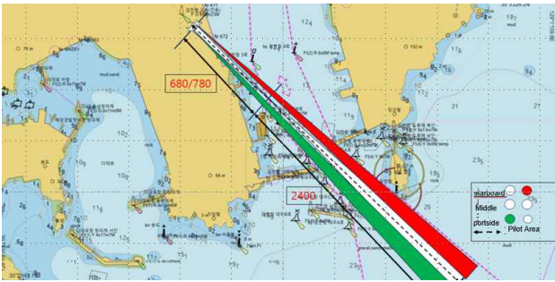
Fig. 3 Estimated installation location(Double Sector Lights)
