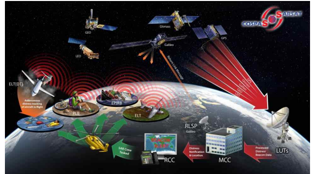
Source : C/S G.003, Cospas-Sarsat, 2022 Fig. 8 Improved Cospas-Sarsat System including MEOSAR
