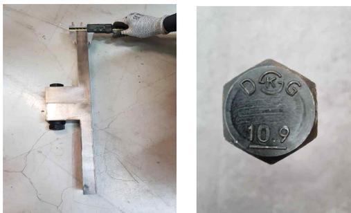
(a) L-type Flange (b) High tension bolt
