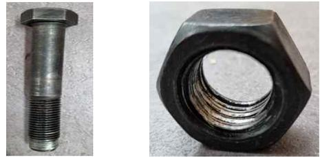
Phot. 4 Wear geometry of bolts and nuts
