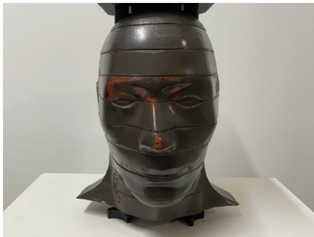
Fig. 2. Distribution of the 9 anatomical slices in the Alderson Rando phantom. Each level corresponds to the site of dosimeter insertion, as described in Table 2.
