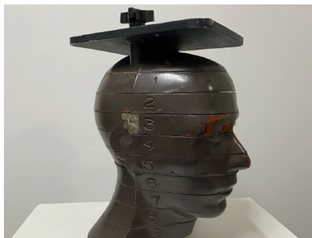
Fig. 1. Alderson Rando anthropomorphic phantom (model ART-200, RSD Phantoms, Long Beach, CA, USA).
