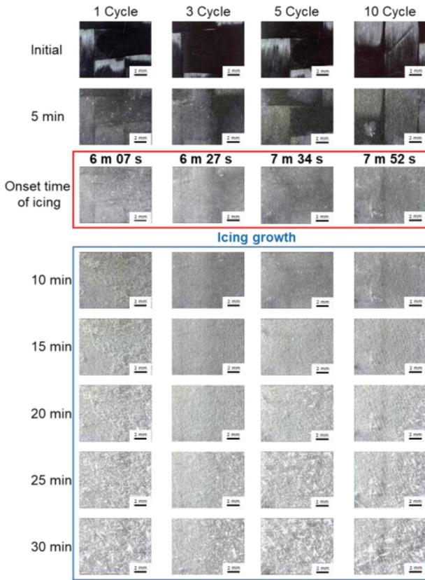
Fig. 2. Photos of onset of icing cycle and icing growth on topcoat surface during de-icing cycle
