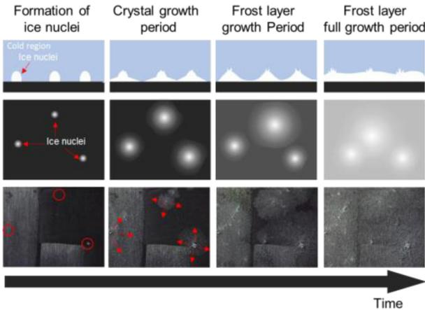
Fig. 1. Frosting mechanism of under ultra-low temperature
