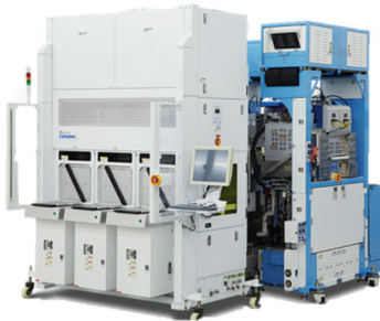
Fig. 1. A PE-CVD System used in the Semiconductor Industry [Source: Wonik IPS].
