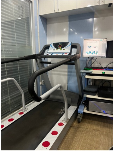
Fig. 2. Treadmill gait analysis was performed using the Zebris Co. Ltd FDM-T system.
