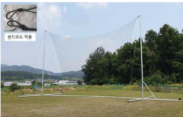
Fig. 14 Net recovery system
