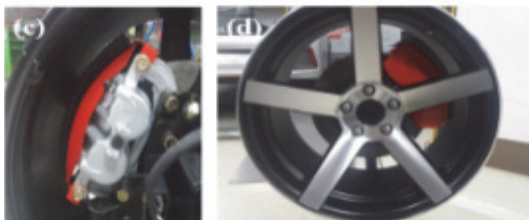
(c) and (d) the dust collector installed in the caliper
