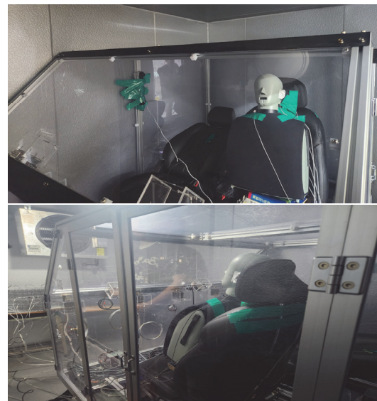
Fig. 3 Human body dummy installed in the chamber
