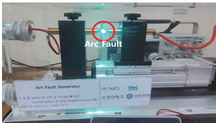
(a) Arc Fault Condition
