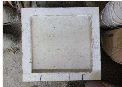
Fig. 4. Scaling test specimen
