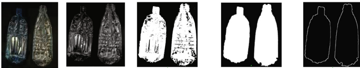
Figure 1: the steps of proposed method for segmenting and classifying a plastic bottle
