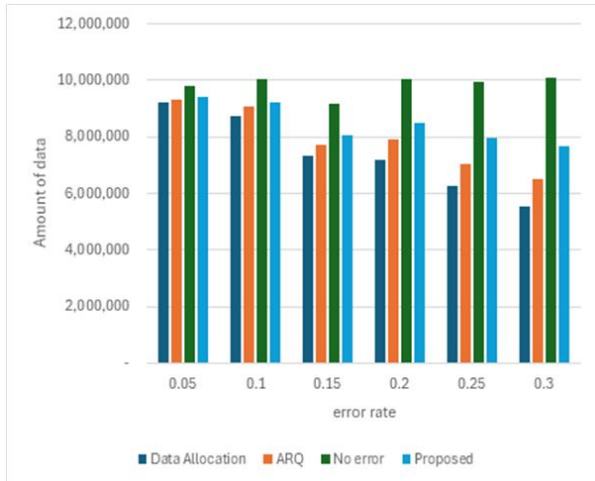
Fig. 5. Comparative Analysis of Data Quantity Received by Sync Nodes with Changes in Error Rates
