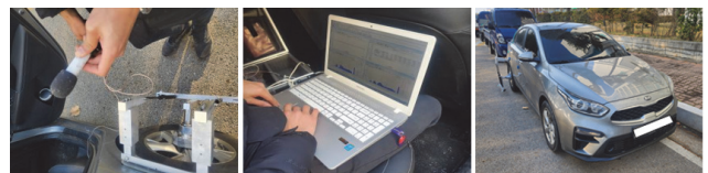
Fig. 5 Traffic noise test(CPX method)
