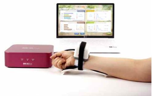
Figure 1. 3-dimensional tonometric radial pulse analyzer(DMP-Lifeplus)
