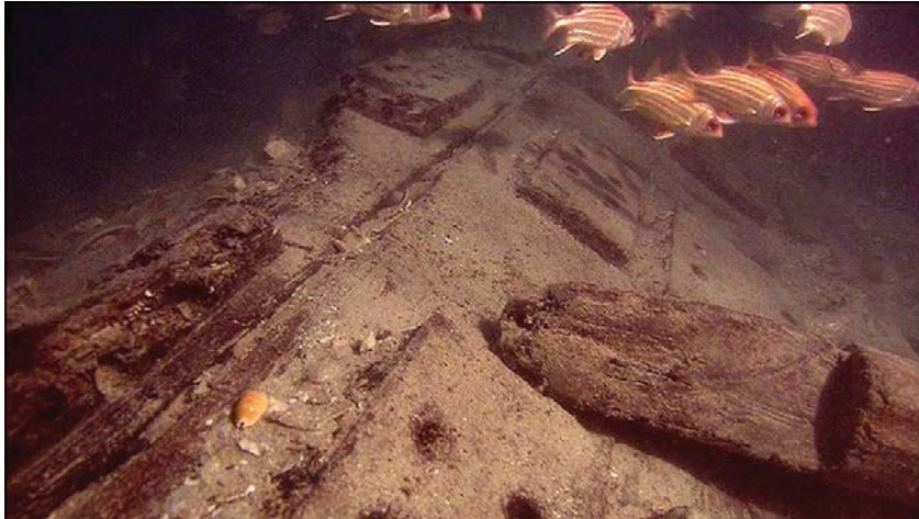
Figure 7. Inner strakes of the Cirebon Shipwreck show protruding rectangular lugs with holes to pass ropes through to fix frames. A robust timber at the right bottom is a part of the frame. Courtesy of Ministry of Marine Affairs and Fisheries of Indonesia.
