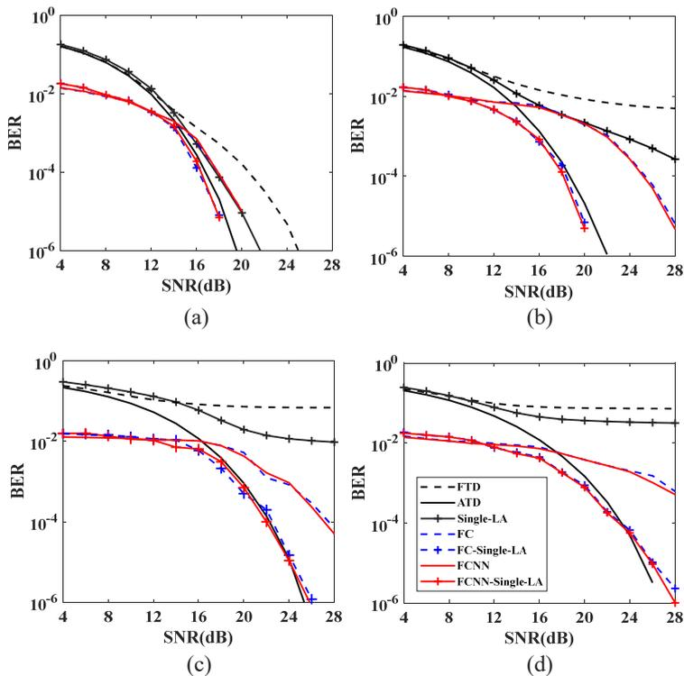
**FIG. 7.** Bit-error-rate (BER) performance of the proposed single logarithmic amplification (LA) and deep learning (DL)-based on-off keying (OOK) detection for optimized  $b$  value: (a)  $\sigma_i^2 = 0.0596$ , (b)  $\sigma_i^2 = 0.1256$ , (c)  $\sigma_i^2 = 0.2080$ , and (d)  $\sigma_i^2 = 0.4286$ .
