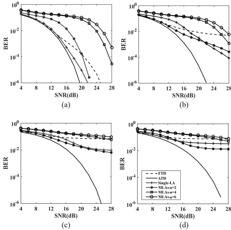
**FIG. 6.** Bit-error-rate (BER) performance of multilevel logarithmic amplification (MLA)-based on-off keying (OOK) detection, under optimized  $b$  value: (a)  $\sigma_i^2 = 0.0596$ , (b)  $\sigma_i^2 = 0.1256$ , (c)  $\sigma_i^2 = 0.2080$ , and (d)  $\sigma_i^2 = 0.4286$ . LA- $n = 1$ , single-LA; MLAs- $n = 2$ , 2-level of MLAs; MLAs- $n = 4$ , 4-level of MLAs; MLAs- $n = 6$ , 6-level of MLAs.
