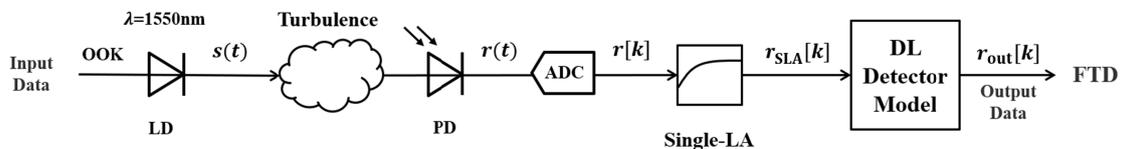
FIG. 1. Block diagram of the proposed technique.
