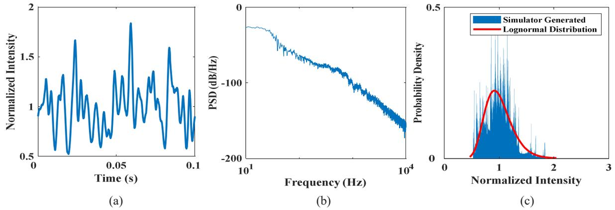
**FIG. 4.** Modeled turbulence channel for  $\sigma_I^2 = 0.0596$ : (a) Time domain, (b) frequency domain, and (c) probability density function (PDF).
