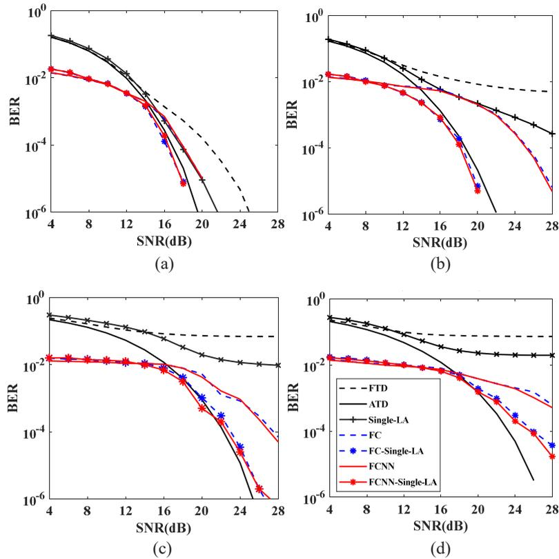
**FIG. 8.** Bit-error-rate (BER) performance of the proposed single logarithmic amplification (LA) and deep learning (DL)-based on-off keying (OOK) detection for fixed  $b$  value: (a)  $\sigma_I^2 = 0.0596$ , (b)  $\sigma_I^2 = 0.1256$ , (c)  $\sigma_I^2 = 0.2080$ , and (d)  $\sigma_I^2 = 0.4286$ .
