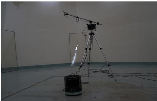
Fig. 1. (Color available online) Example of the measurement setup for calibrating the reference sound source.
