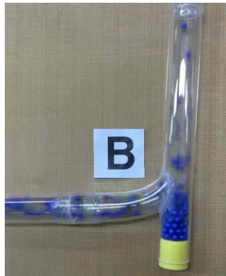
Fig. 13. Replacement samples piled up in a T type pipe
