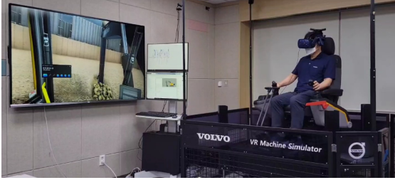
Fig. 4 Excavator simulator by RT simulation
