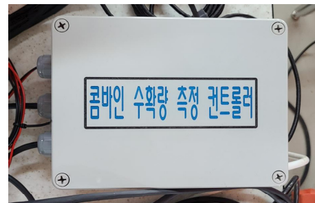
Fig. 10 Main controller of rice yield prediction system (a) design (b) main controller
