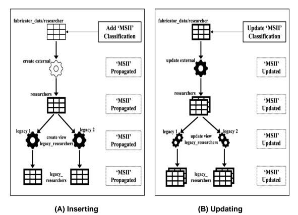
Figure 2. Inserting& Updating metadata schema identification information (MSII) repository propagation using Fabricator.
