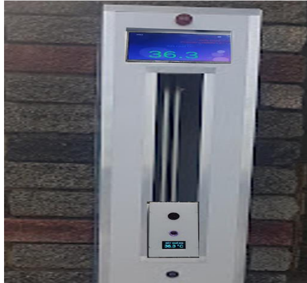
Figure 7. Measured result display on both of LED screen and LCD screen
