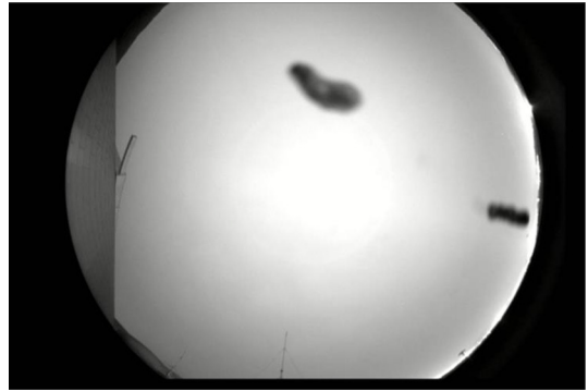
Fig. 5. An all-sky image with small materials, though to be branches, on its camera. Even though it was a cloudy night, the all-sky image is misclassified as “Not Cloudy” via our machine learning model.
