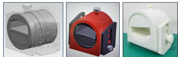
Fig. 3. The developed aid fabricated by 3D modeling design using a 3D printer.
