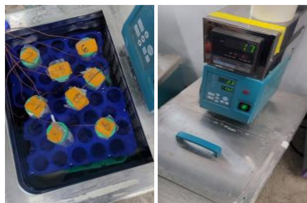
Fig. 2. Exotherm analysis (Left, samples; Right, refrigerated circulating water bath with programmable temperature controller).
