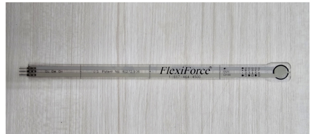
Fig. 3. Force sensing resistor used in this study (Flexiforce A201 sensor)
