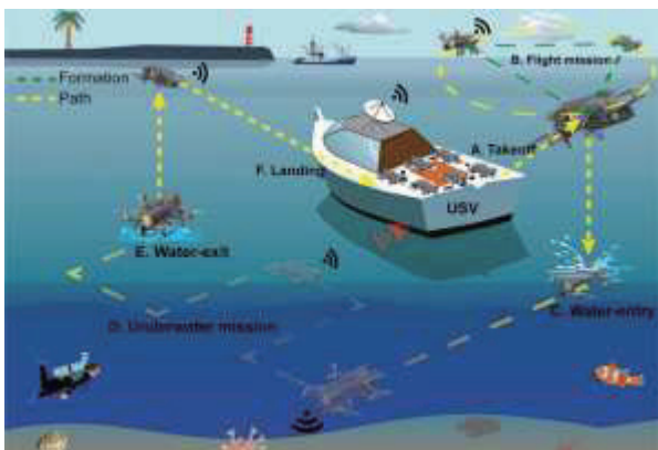
Fig. 1 Concept of UAV/USV Cooperative Operation [4]
