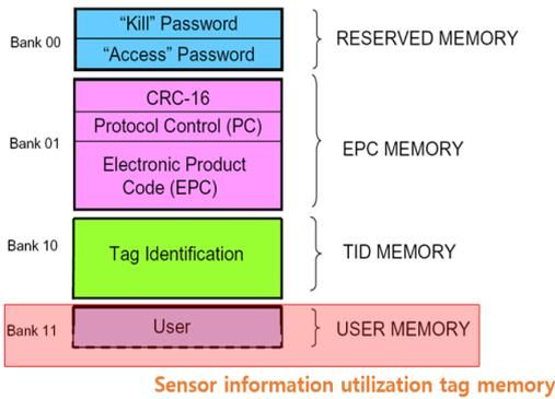
[Fig. 5] Smart tag memory recognition structure diagram
