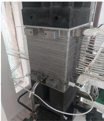
Fig. 1. Photograph of 30-cell H<sub>2</sub>O-CO<sub>2</sub> SOEC stack
