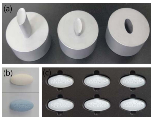
Fig. 1. Comparison of the standard sample tableting of the lab-produced and commercial-scale-produced tablets. (a) Tableting parts for producing the standard samples. (b) Comparison of the manufactured standard sample tablets and commercial-scale-produced tablets. (c) Dedicated tray for the Raman measurement.
