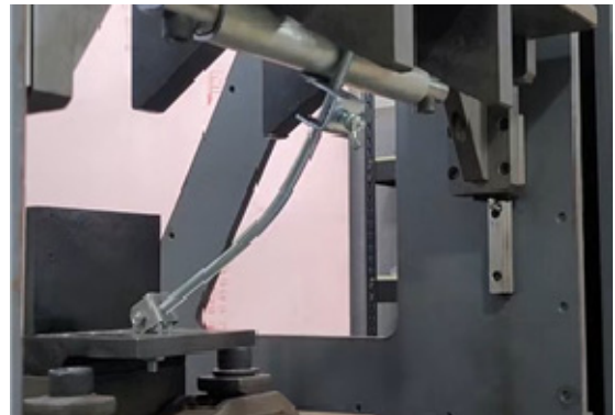
[Figure 2] Buckling of Eccentric Type 2-1
