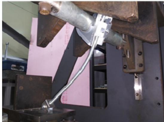
[Figure 4] Buckling of Eccentric Type 2-3
