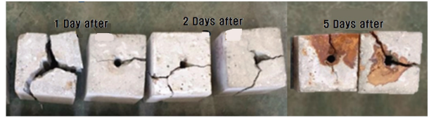
Fig. 10. Corroded samples after bond strength test
