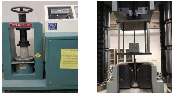
(a) Compressive test (b) Pull-out test Fig. 5. Test of compressive strength and pull-out test
