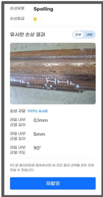
(a) External diagnosis results of rail surface damage
