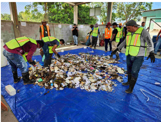
Fig. 1. Waste sampling through out conical quartering method.
