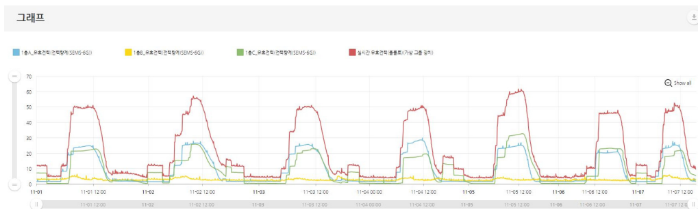
Fig. 4. Real-time active power monitoring (based on the load of three distribution boards)
