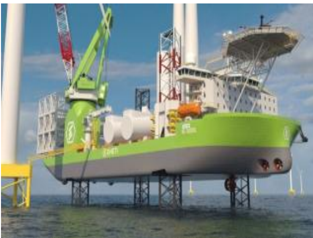
Fig. 1. A example of the elevating wind turbine installation vessel ( https://www.splash247.com ).
