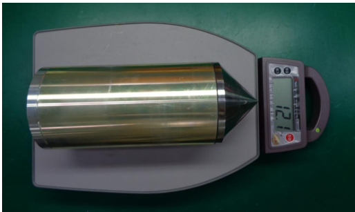
Fig. 3. Geometry and weight of bird assembly
