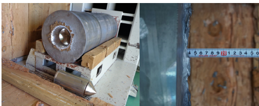
Fig. 4. Crater geometry and depth after test
