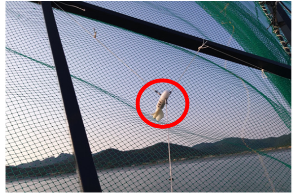
Fig. 4. Flow meter attached to the shrimp dredge fishing gear to estimate biomass of Metapenaeus joyneri used flow quantity in the coastal water of Gochang, Jeollabuk-do, Korea from May to Sep. 2021.
