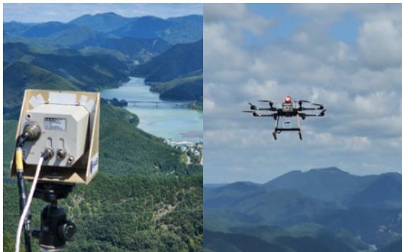
Fig. 4. Tripod(left) and UAV(right) mount on MAW-400
