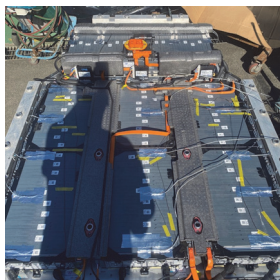
Fig. 1 The layout of LIB modules and location of sensor in pack
