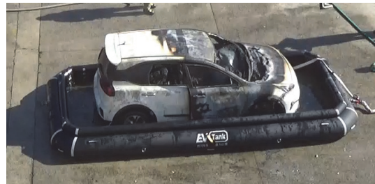
Fig. 8 Completion of EV vehicle fire suppression
