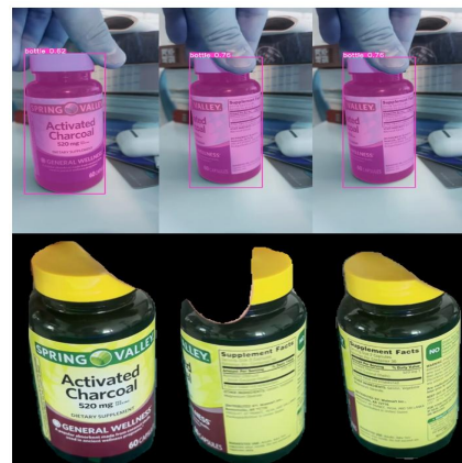
Fig. 2. Yolov8 Pill bottle segmentation
