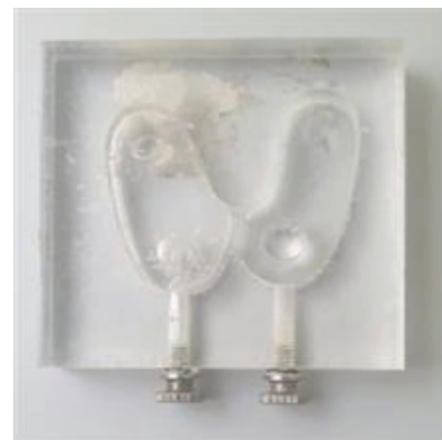
(a) Thyroid Phantom (Thyroid Phantom 128-340, NucleMed, BE, 9.25 MBq)
