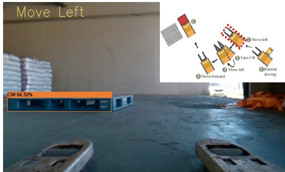
(a) Center misalignment, command: Move Left
